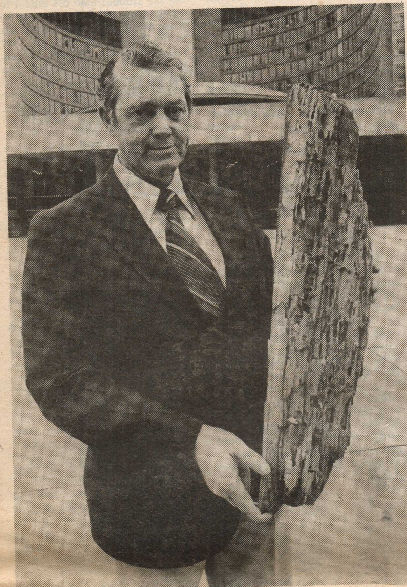
City of Toronto Termite Control Officer Bob Lott holds remains of fence post destroyed by termites. Resembling a grain of rice in both size and colouring, termites live on cellulose obtained from eating wood or wood-based products. Homeowners in the City can obtain counselling and financial assistance towards treatment of termite infestation by calling 469-2358.
