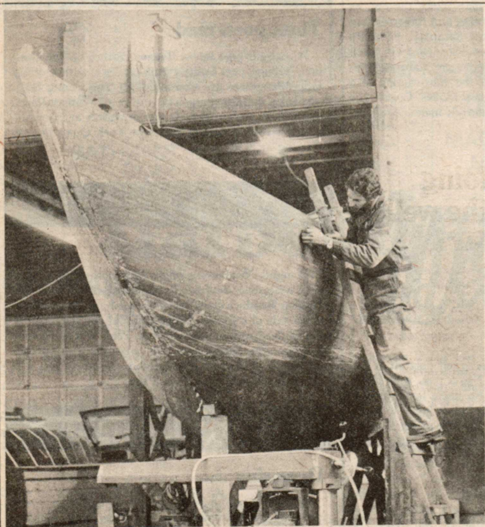
Wooden boats get a second chance . . . Boatbuilder Nial Leslie works on the restoration of an 8-metre at the Canadian Shipwright Guild.
