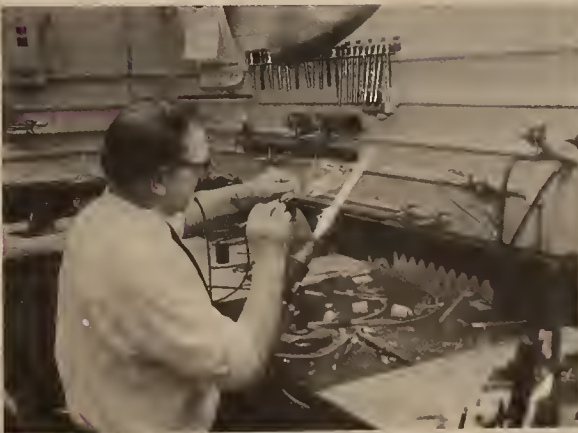
The University has three glass-blowers who make most of the complicated glass equipment for the chemistry department. Here chief glassblower Jahn French is farming a flask on his lothe. It takes 15 years to train the kind of all-round artisan needed for this work. It takes only four years to get a B.A.
